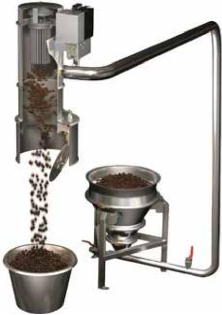
Pneumatic conveyors transfer powder or granules within processing or manufacturing machinery in selected quantities and within desired time. The transfer of materials takes place in perfect hygienic condition, respecting both the environment and the operators' health.
