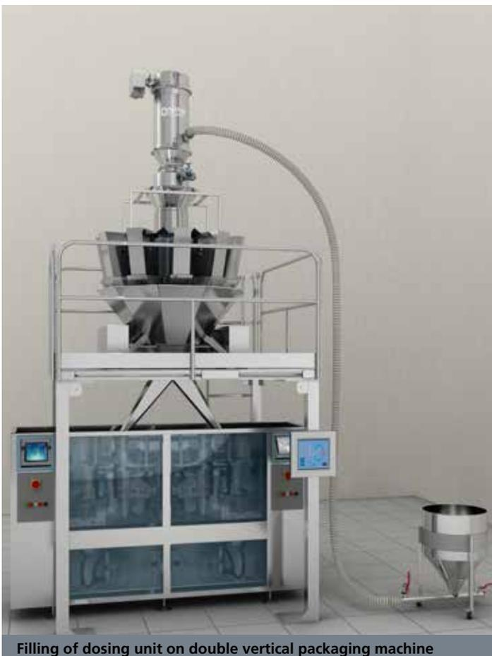
Filling of dosing unit on double vertical packaging machine
